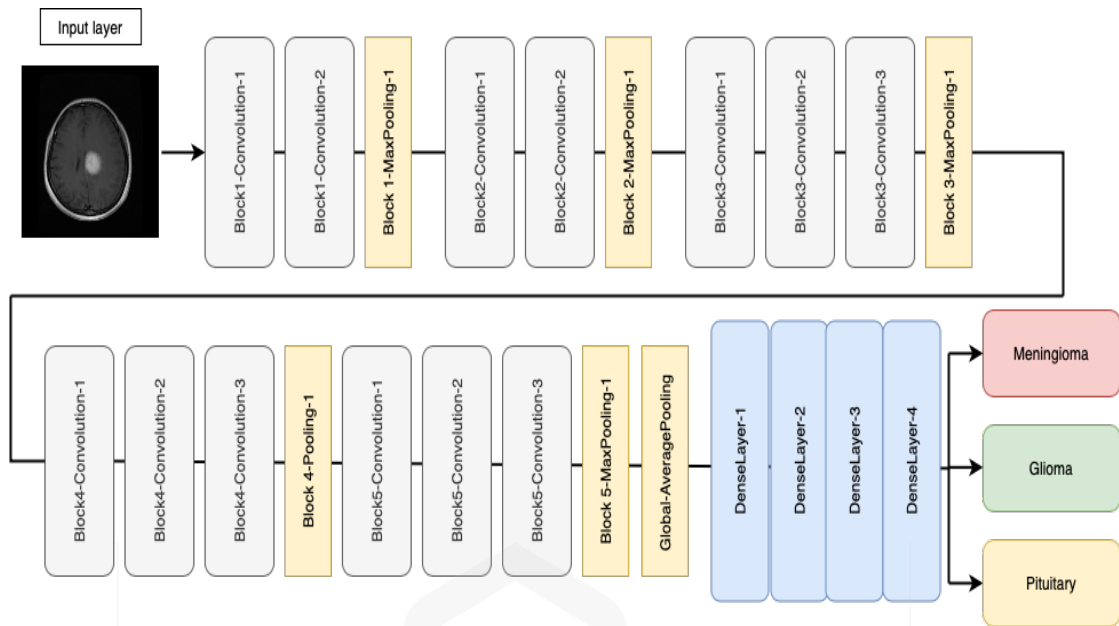
Figure 4.8 Transfer learning of VGG16 for multiclass classification task
