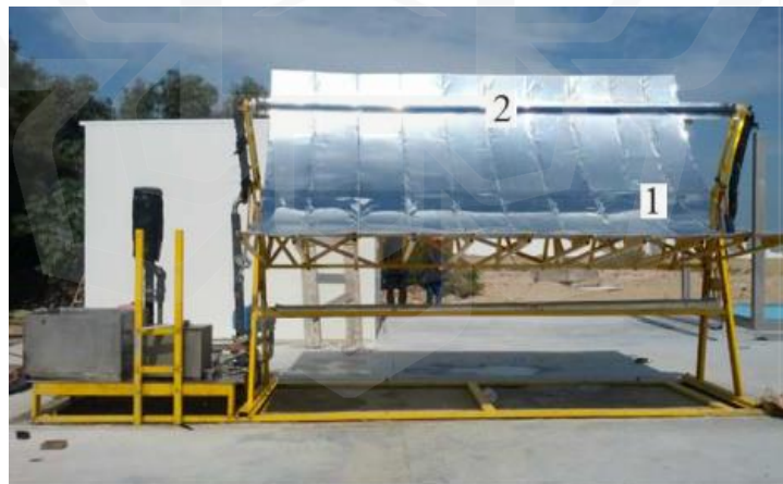
Figure 2.5: Parabolic Trough Collectors (PTC) (1) reflector, (2) receiver (Chafie et al., 2018)
