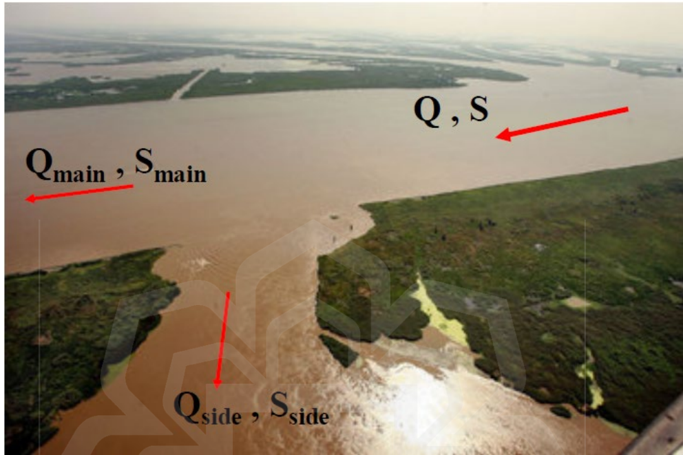
Figure 1.1 Mississippi River ( Q, S ), its West Bay diversion ( Q_{\text{side}}, S_{\text{side}} ) and downstream reach ( Q_{\text{main}}, S_{\text{main}} ). (Dutta, 2017)
