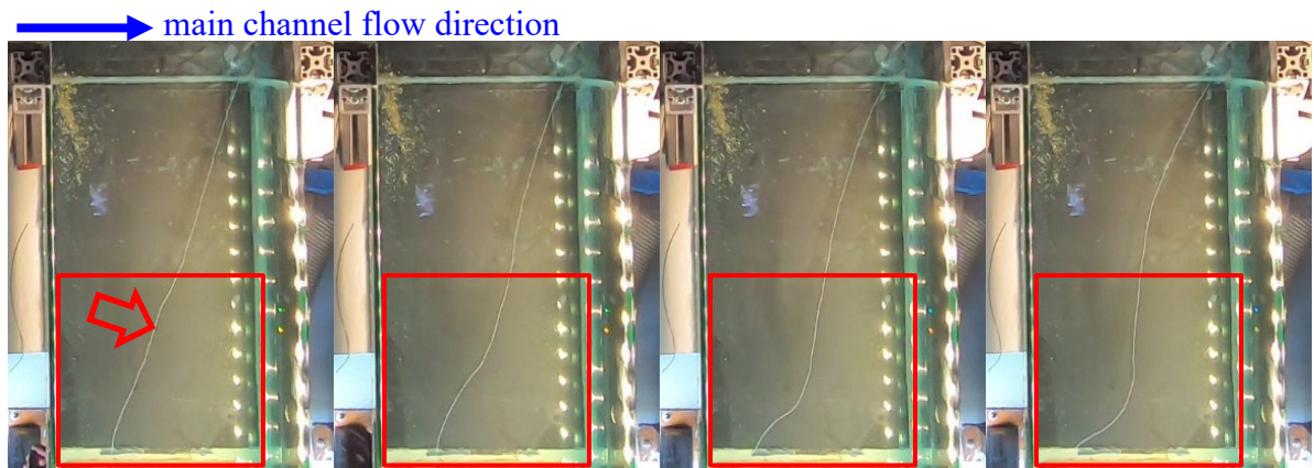
Figure 3.8 GoPro video snapshots of white thread movement (in four 1-second frames) for Trial 7 (Table 3.4) – 2D standard closed recirculation (Figure 3.6)
