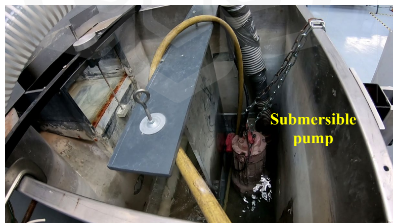
Figure 3.3d Photos of experimental setup – downstream tank, weir and submersible pump
