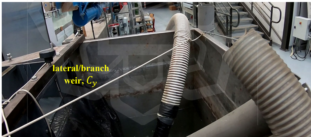
Figure 3.3c Photos of experimental setup – lateral/branch tank and weir
