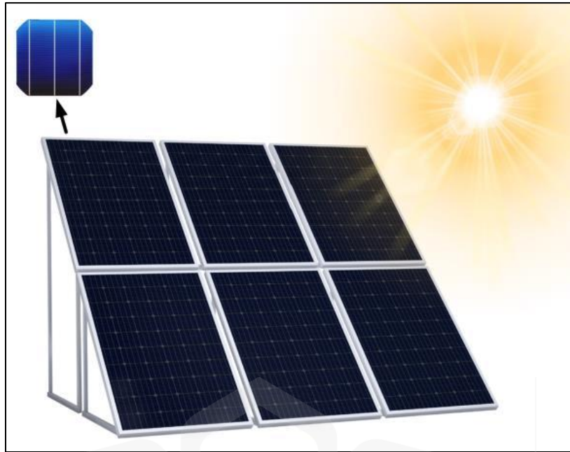
Figure 2.7 Solar PV Array (Duranay, 2023)
