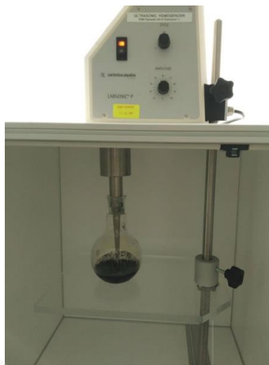
Figure B.14: Immobilization of MWCNT
