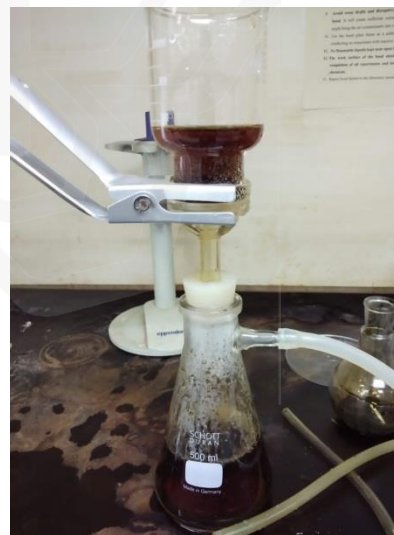
Figure B.12: Filtration of functionalized MWCNT
