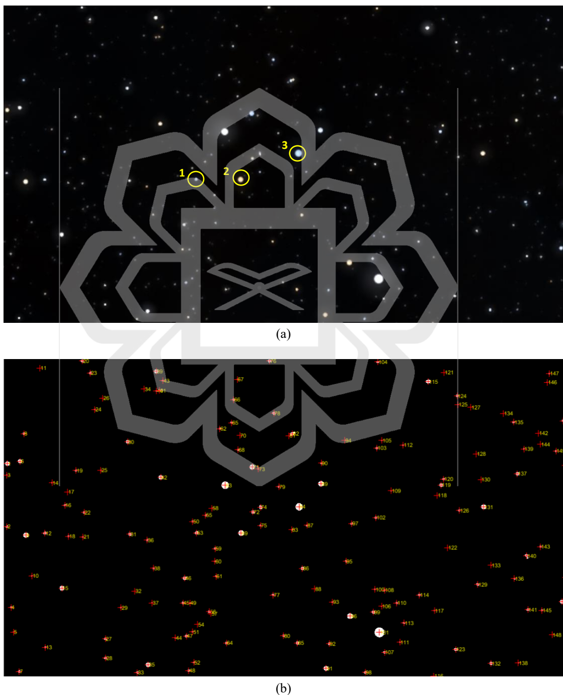
Figure 4.13: (a) Star field of Image 2-4 with an SNR of 0.27 dB. (b) Centroid positions of all detected stars.
