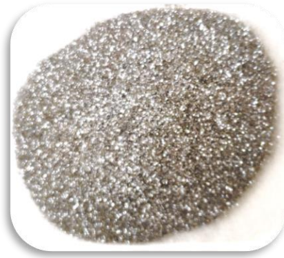
Figure 3.2 Ti coated diamond powder as reinforcement material
