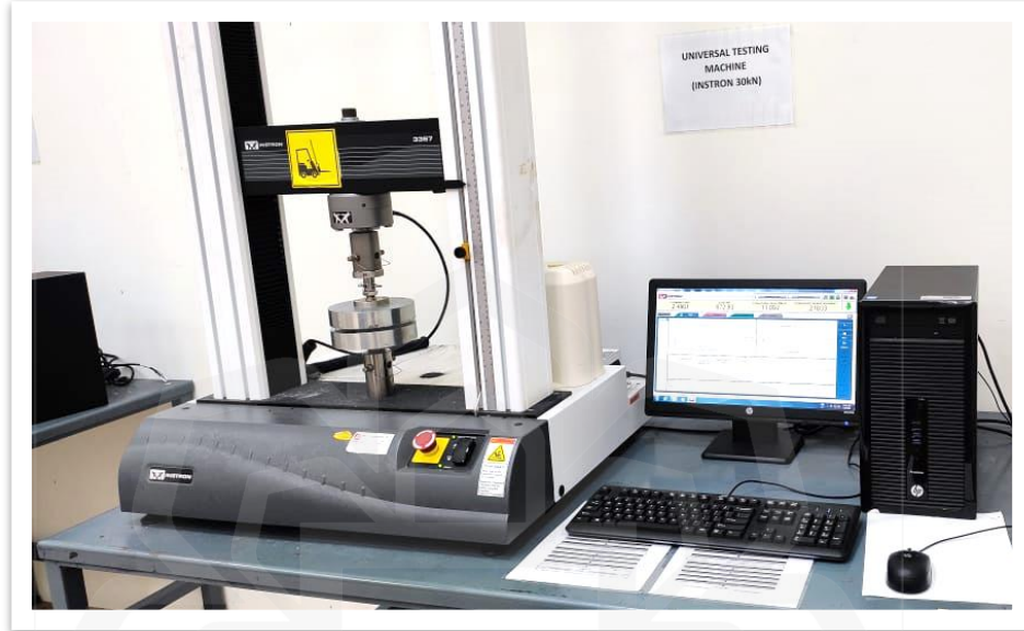
Figure 3.11 Compression testing machine with 30 kN load
