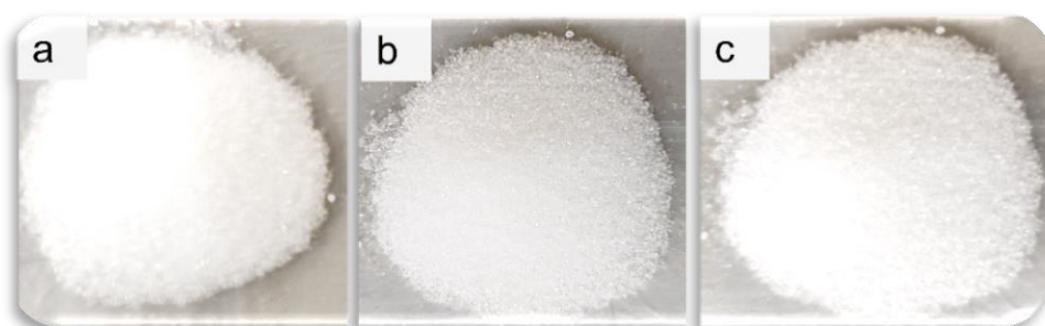
Figure 3.3 Various sizes of PMMA particles, (a) 75 \mu\text{m} , (b) 125 \mu\text{m} , and (c) 150 \mu\text{m}
