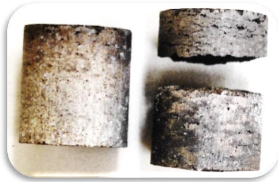
Figure 3.7 Sectioned samples from porous Al composite
