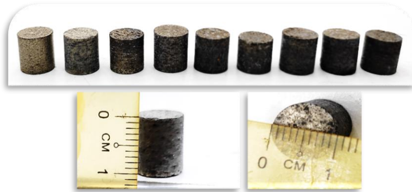
Figure 3.6 Sintered samples of size 10×10mm
