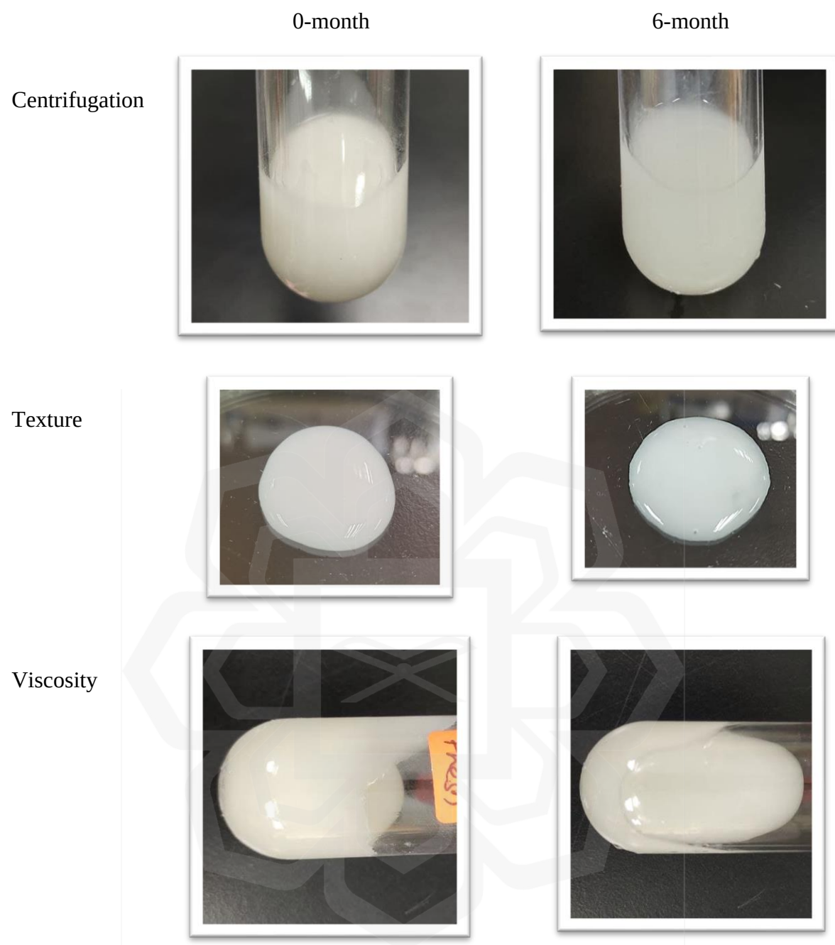
Figure 3.2 Centrifugation, Texture and Viscosity Observation of the Gel-Cream Formulation
