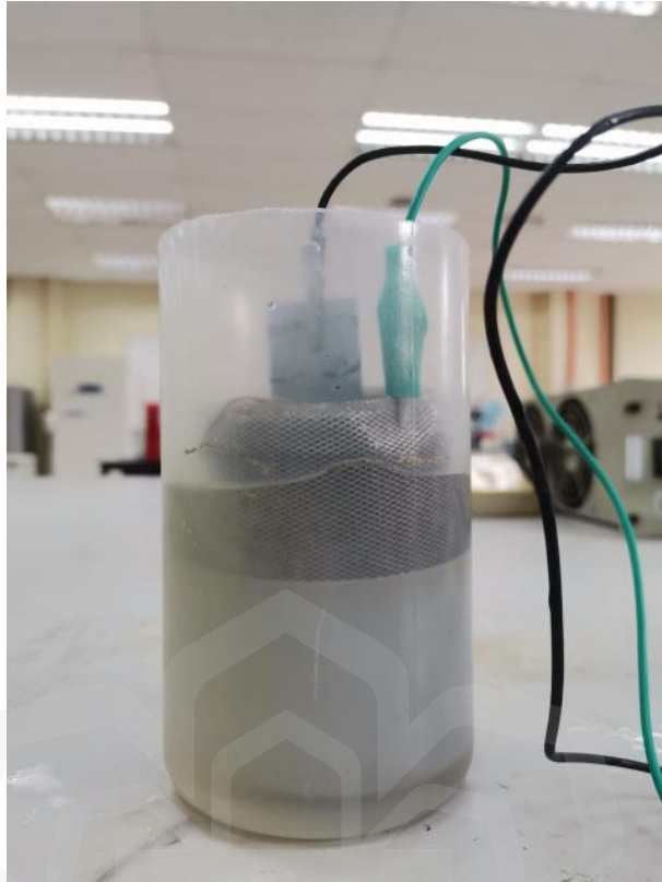
Figure show setup for zinc/air MFC with fabricated air cathode
