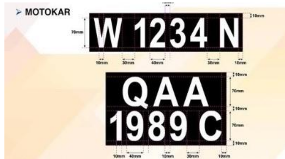
Figure 1.2 The Two Types of Orientations of LP in Malaysia with Standardized Specifications
