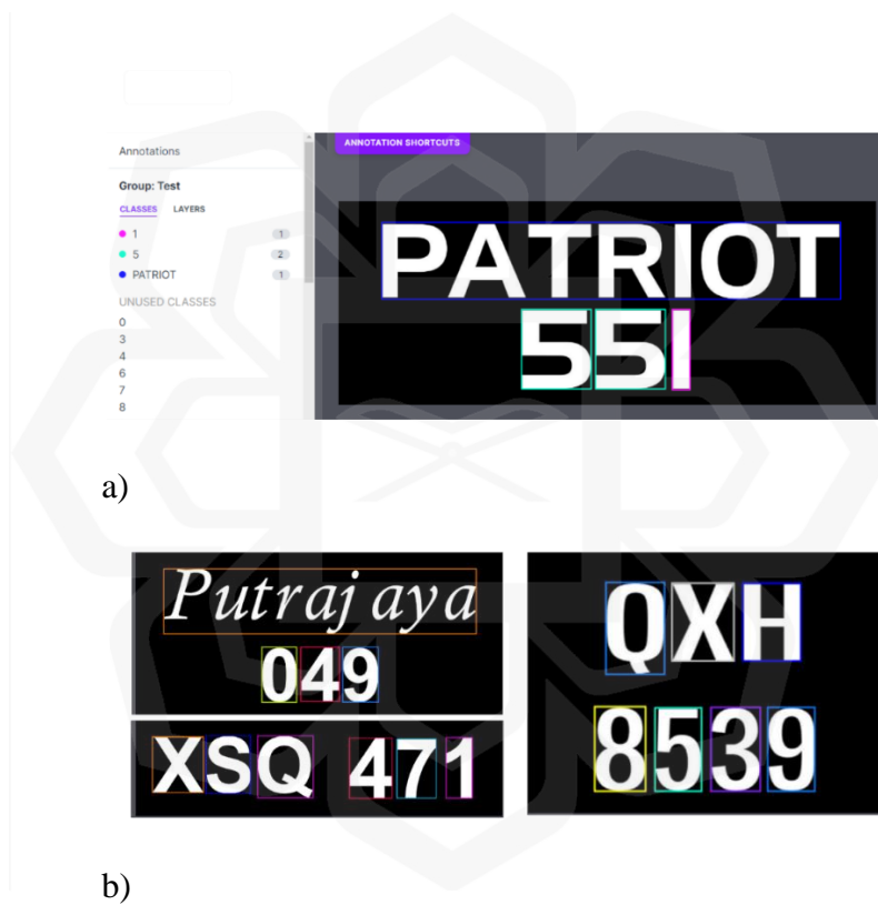
Figure 3.11 Labeling the Synthetic Dataset ideally, a) Labels with Classes Visualized in Roboflow, b) Samples of Different Layout LPs Labeling.
