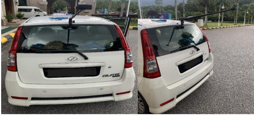
Figure 3.2. Installed Camera Setup on the Survey Vehicle
