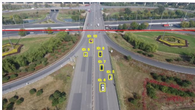
Figure 2.15 Vehicle Tracking Results using Aerial Video (Xiang et al., 2018)
