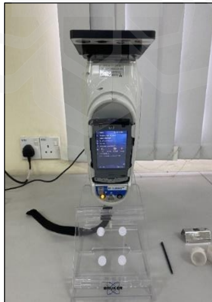
Figure 3.10 Bruker S1 Turbo SDR Portable XRF Spectrometer X-ray Fluorescence SDD.
