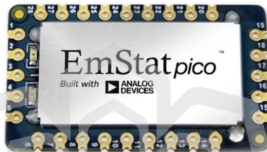
Figure 2.24 Packaging of 1.1.1 EmStat Pico Core (PalmSens BV, 2023)
