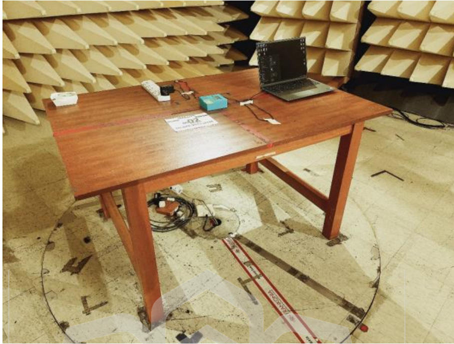
Figure 4.17 Radiated emission and radio-frequency electromagnetic field setup.
