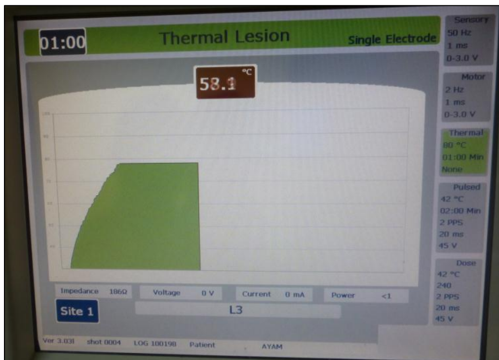
Figure 5.3: Rate of temperature increase for existing cannula
