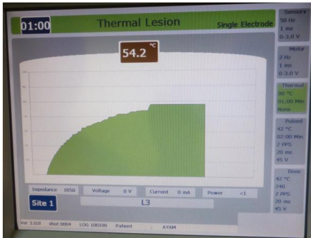
Figure 5.4: Rate of temperature increase for prototype cannula
