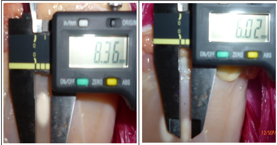
Figure 5.1: Width lesion shape dimension for prototype cannula and existing cannula respectively
