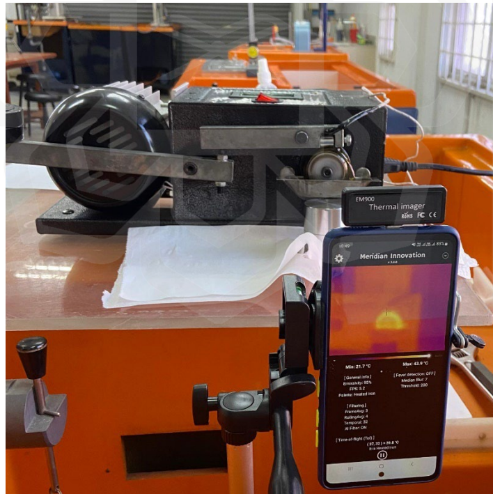
Figure 3.4 Thermal camera set up to monitor interface temperature
