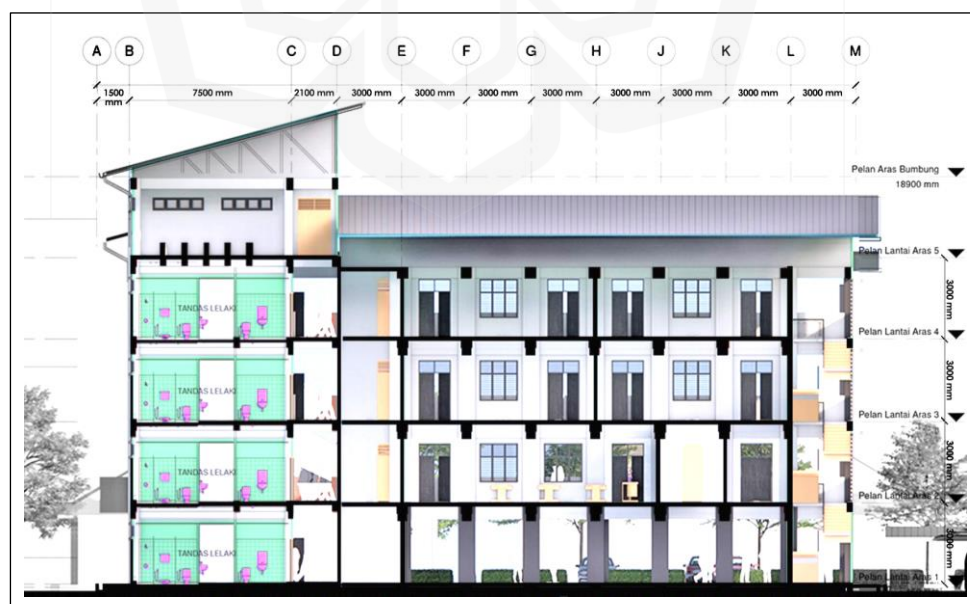
Figure 2.3 Typical Block Section
