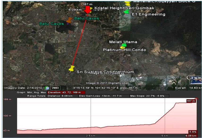
Figure 3.29: Location and path profile of 6 km sites viewed in Google Earth Configuration of test setup for the 6 km test is as presented in Figure 3.30
