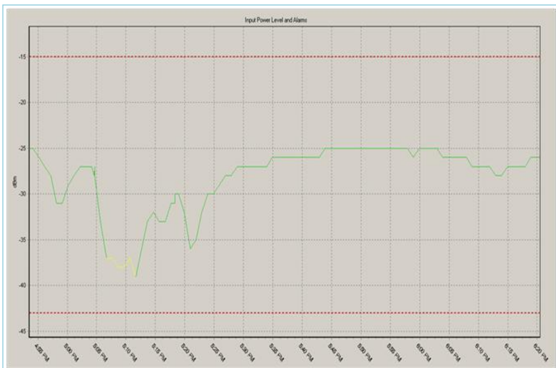
Figure 3.5. Sample of attenuation of FSO link during rain on 2 October 2011
