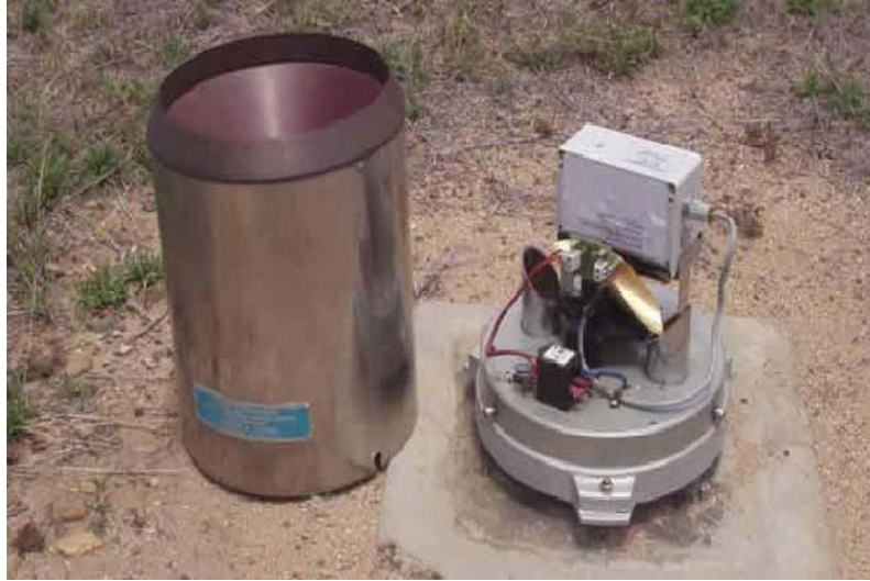
Figure 3.14: MMD Tipping Bucket at KLIA
