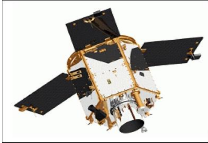
Figure 3.4: RazakSAT with Solar Panel Deployment
