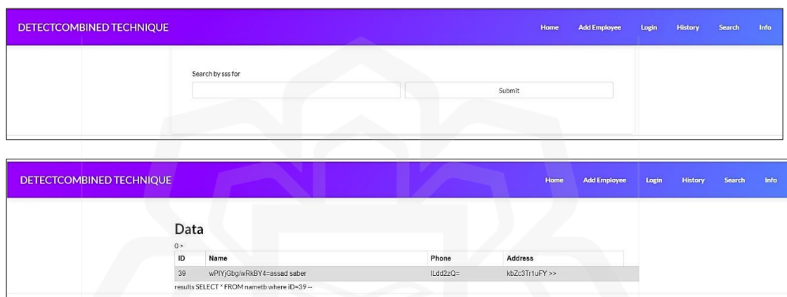
Figure 4.16: The search result with protection against SQL injection
