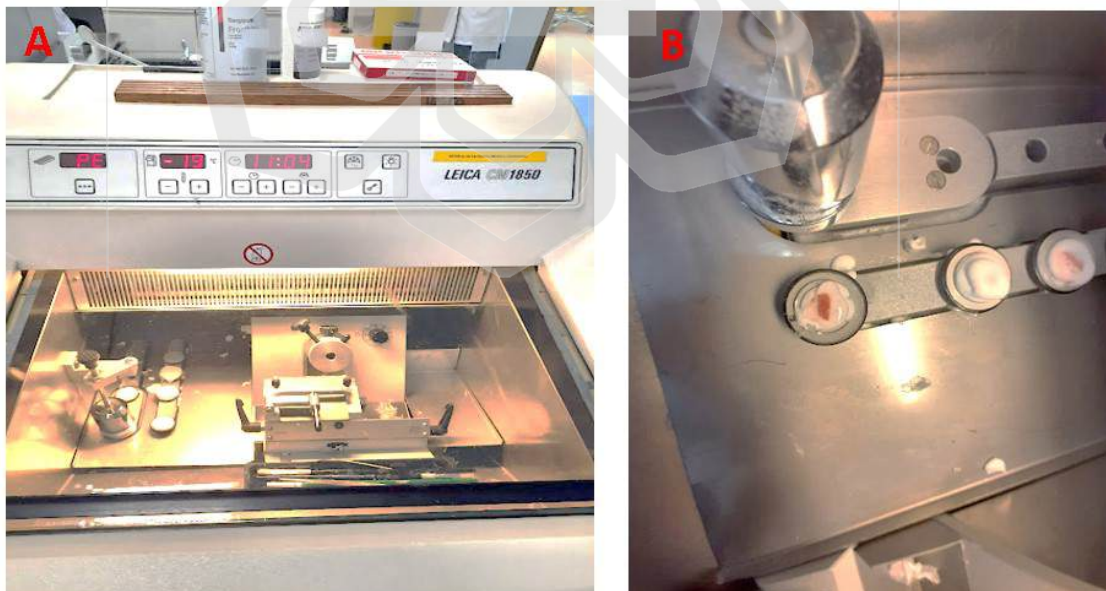
Figure 3.16 Cryostat Chamber with Cryomould Inside (A), Close-Up View Cryomoulds Inside the Cryostat Chamber (B).
