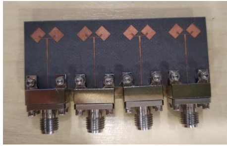
Figure 5.5 The Fabricated Proposed 1 x 4 \pm 45^\circ Dual-Polarised Antenna Array (Substrate Thickness of 1.575 mm)
