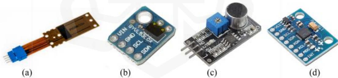
Figure 3.1: Mechanomyography Transducer: a) Piezoelectric contact sensors b) Laser distance sensors c) Condenser microphones d) Accelerometers (N. Li et al., 2024).
