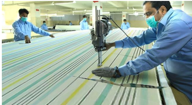
Figure 12.1 Automated cutting process of knitted garments
