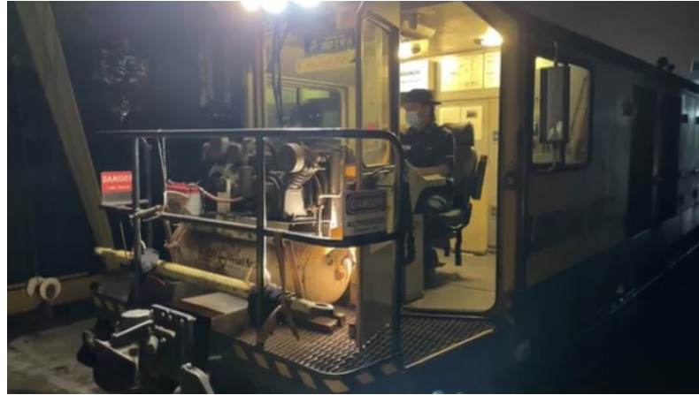
Figure 3.12: LORAM Rail Grinding Unit.
