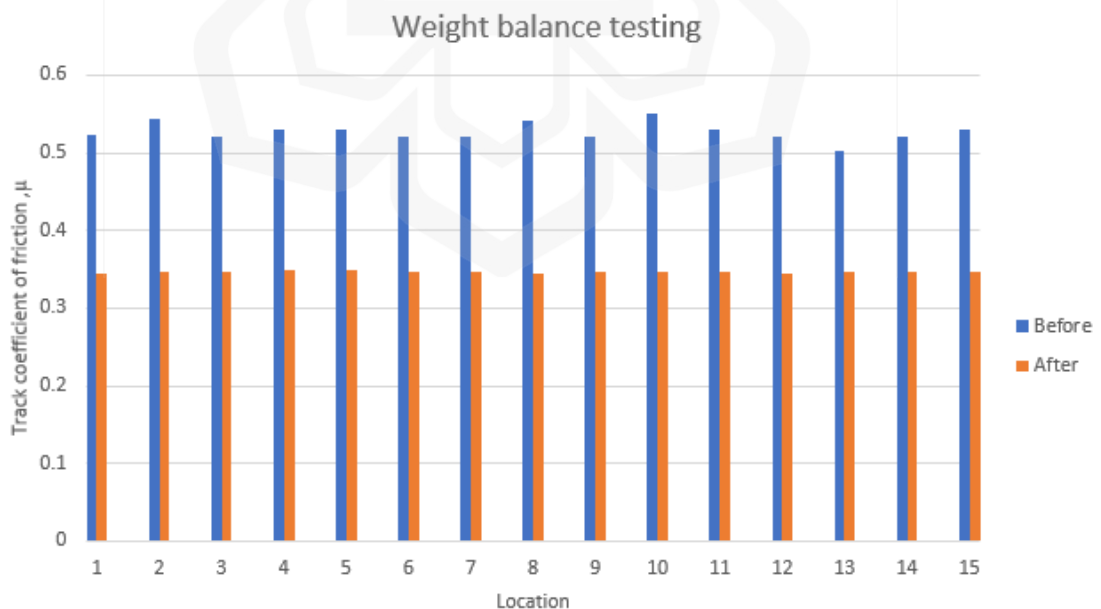
Figure 5.2: Graph of weight balance testing for before and after the application of rail grinding to find \mu .
