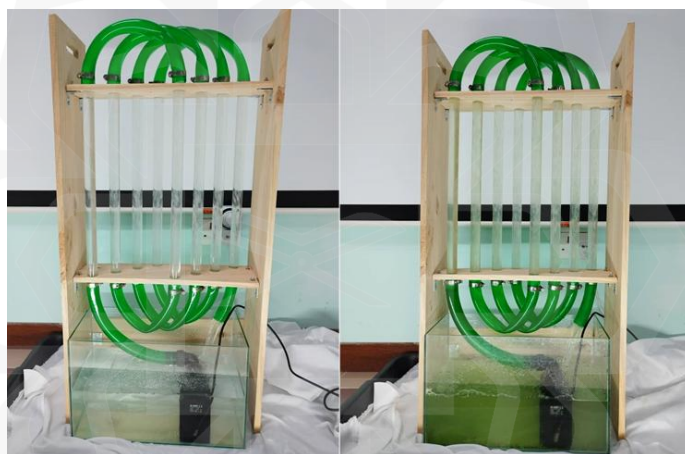
Figure 4.98 Vertical tubular prototype setup from day 1 (left) to day 14 (right)
