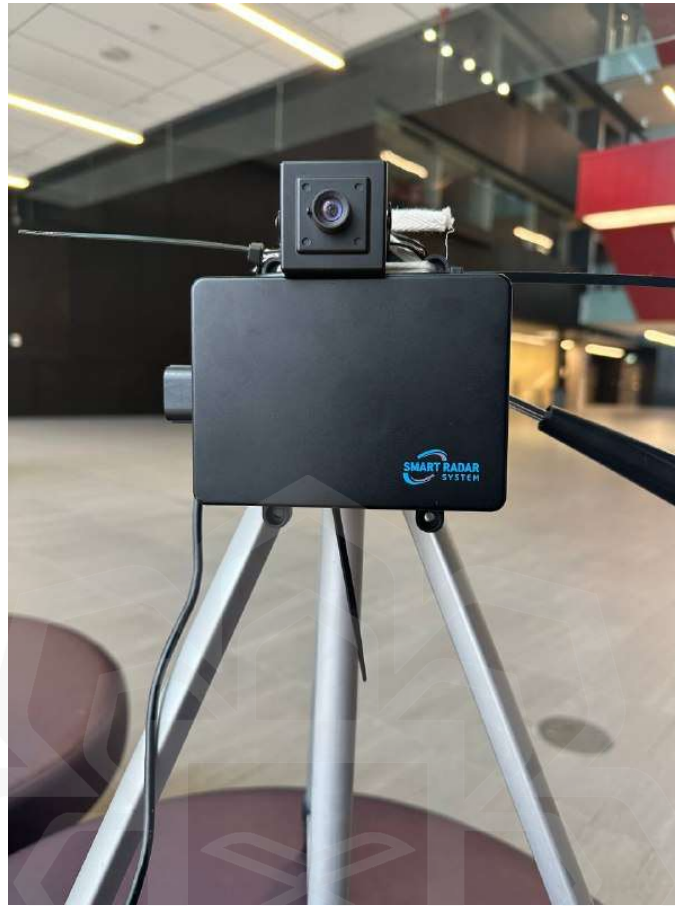
Figure 3.6 Radar and Camera Mounting Arrangement
