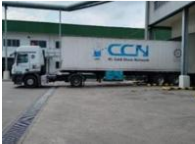
Figure 4.7 Vehicles equipped with a closed cooling system (chiller) for transport and distribution of chicken meat
