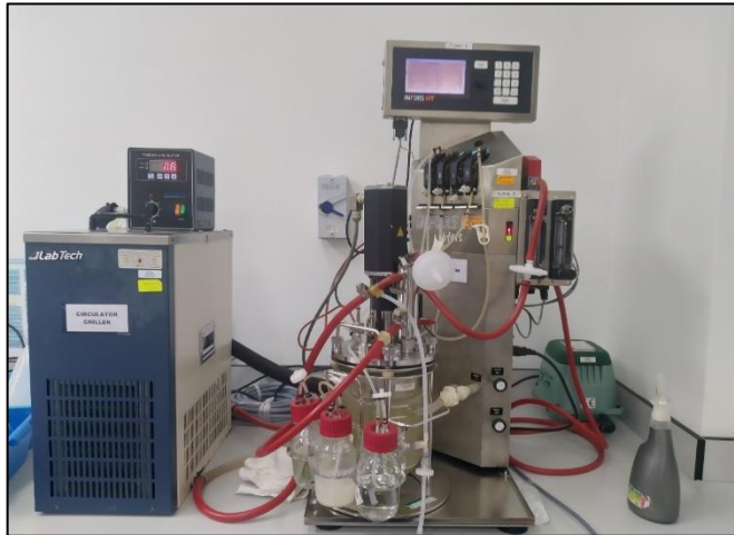
Figure 3.6 Setup of the 2 L bioreactor, Labfors, INFORS HT, Switzerland
