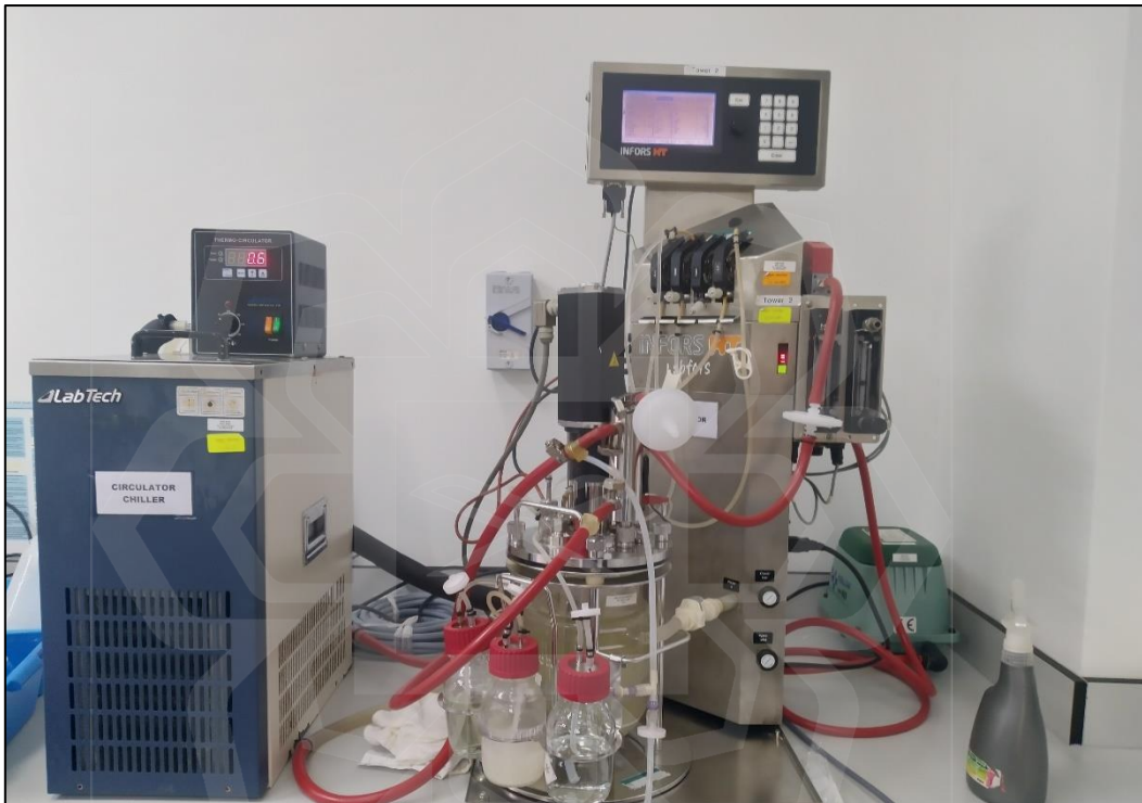
Figure 5.1 Setup of the 2 L bioreactor, Labfors, INFORS HT, Switzerland
