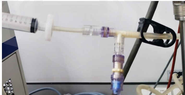
Figure 5.5 Super Safe Sampler for aseptic sampling, INFORS HT, Switzerland
