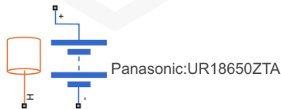
Figure 3.2 MATLAB Simscape Battery (Table-Based) block used for lithium-ion cell modeling. Adapted from MathWorks, 2024.
