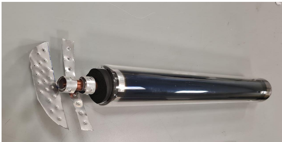
Figure A4-4: Heat Pipe Evacuated Tube Collector (HP ETC) prototype used for air heating application
