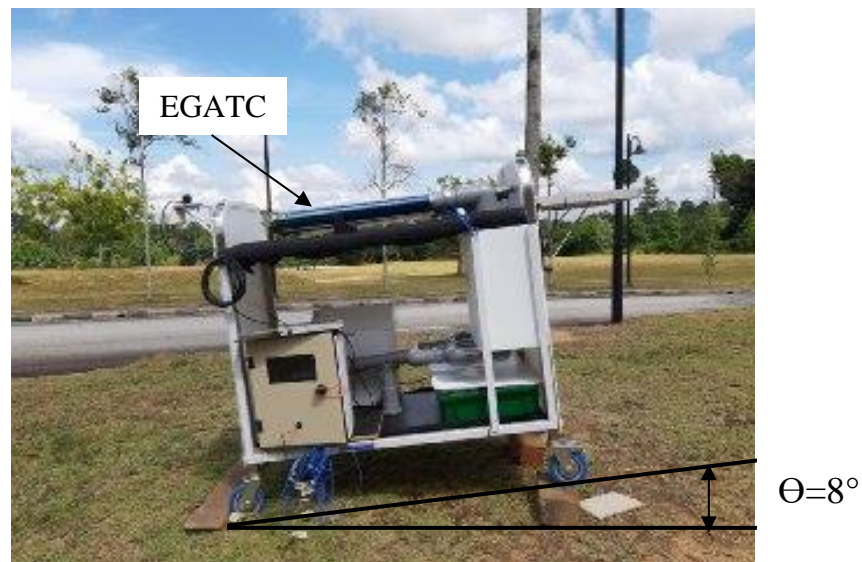
Figure 4.7: The outdoor experiment conducted to determine the effect of the slope angle
