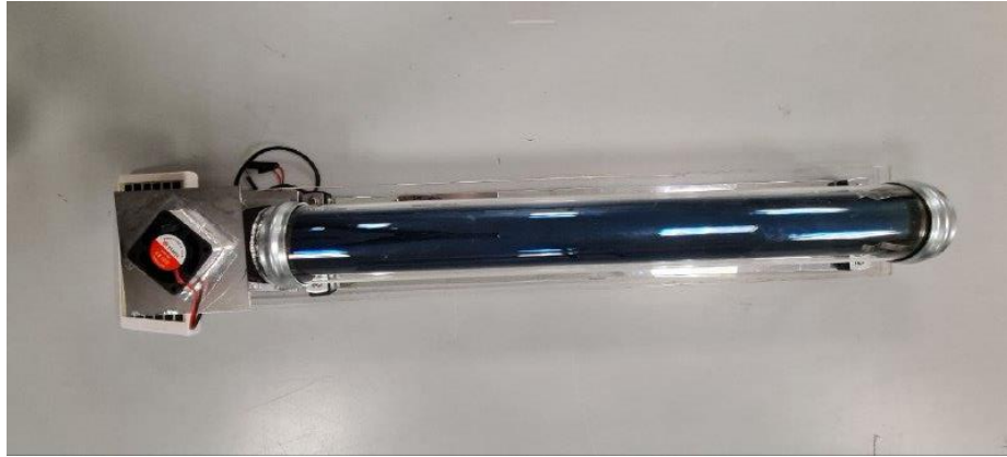
Figure A4-1: Top view of Evacuated Glass- Thermal Absorber Tube Collector (EGATC) prototype
