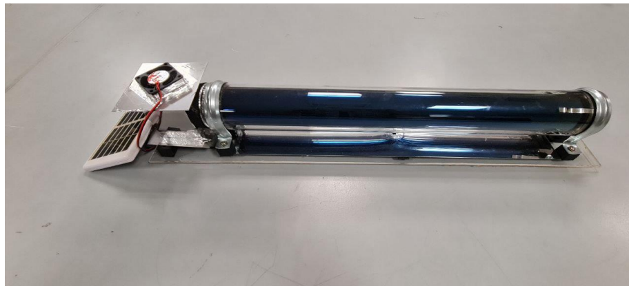
Figure A4-2: Side view of Evacuated Glass- Thermal Absorber Tube Collector (EGATC) prototype
