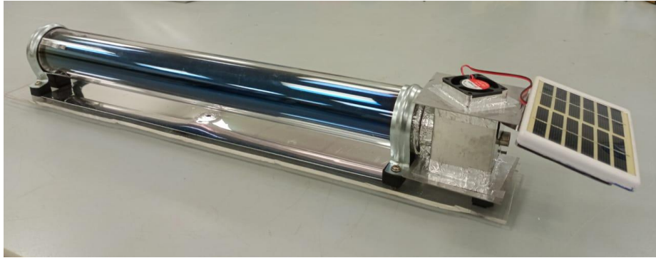
Figure A4-3: Evacuated Glass- Thermal Absorber Tube Collector (EGATC) prototype used for air heating application
