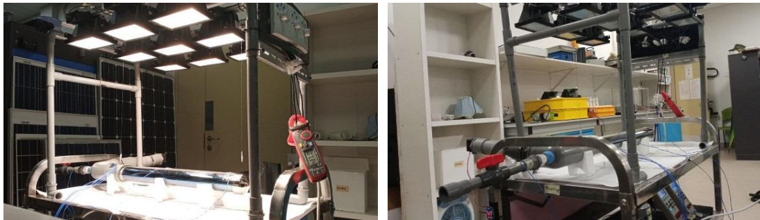
Figure 3.14: The double pass flow experiment of zero (0) fin (insulation material inner absorber) EGATC during charging and discharging
