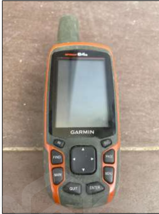
Figure 3.8 Garmin 64s consists of a high-sensitivity GPS with features of a 2.6" sunlight-readable colour screen. It can share wirelessly with other compatible devices on routes, geocaches and waypoints.
