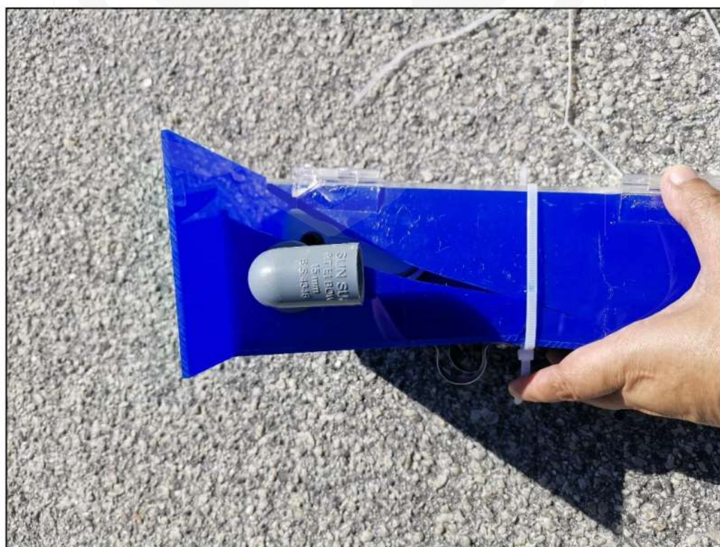
Figure 14. Cover lid equipment broken
